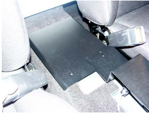
Position rear-floor panel, continue to align with OEM floor nutserts (Item 6)
